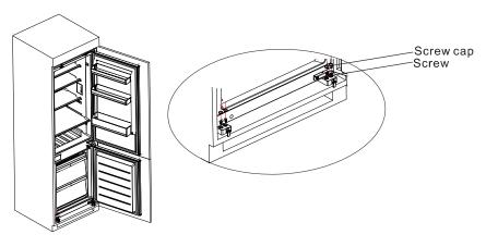
• Fix the top baffle to the top of the cabinet inner with screws, then install the screw caps.
