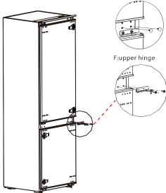
7) Remove the freezer door, the bottom hinge and the hole caps.
