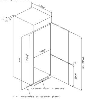
• Push the refrigerator into the cabinet and adjust it to make sure the edge fold of top baffle completely touch the top edge of the cabinet, and the limit hook of supporting leg completely touch the bottom edge of the cabinet.
